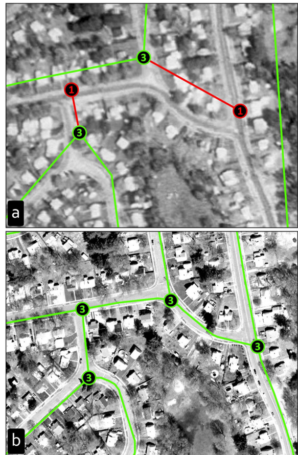
Fig. 1 Street network shape file data and aerial imagery from Connecticut. a Available street network data from 1990 and aerial imagery from 1990 for a neighborhood in Connecticut. b The same location with street network data from 2003 and aerial imagery from 2004. Overall, in a , the street network data are poorly registered with the layout of the streets seen in the aerial images. The red street segment lines and intersection nodes indicate instances where the network data does not reflect the connectivity of the streets shown in the aerial imagery and standard GIS tools for measuring intersection density would produce incorrect results. Analyses of the 1990 street network shape file would identify two, three, or more way intersections in 1990, while analyses of the 2003 shape file would identify four such intersections, which is consistent with the 1990 aerial imagery. The higher spatial and network connectivity accuracy of the more recent street network shape file may provide more accurate estimates of intersection density for an earlier time period, than a shape file from the earlier period
