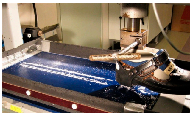
Figure 2. The dynamic coefficient of friction (DCOF) measuring method.
