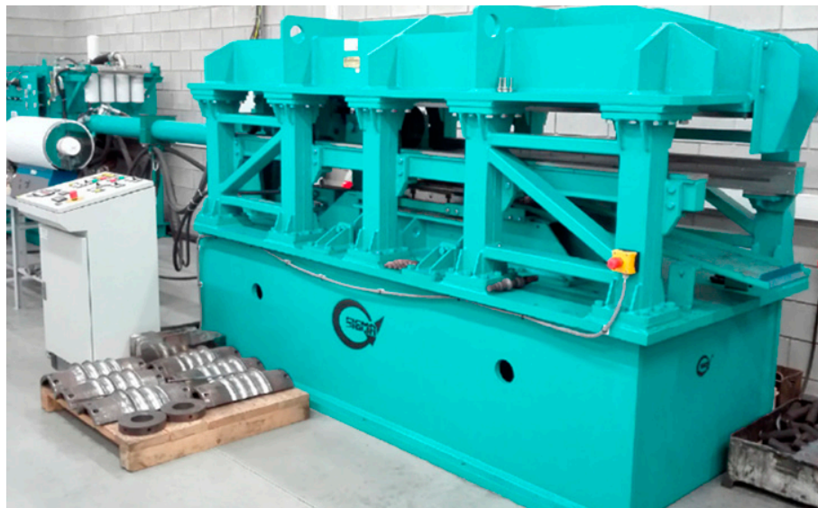
Figure 2. Cross-wedge rolling mill used in experimental testing.
