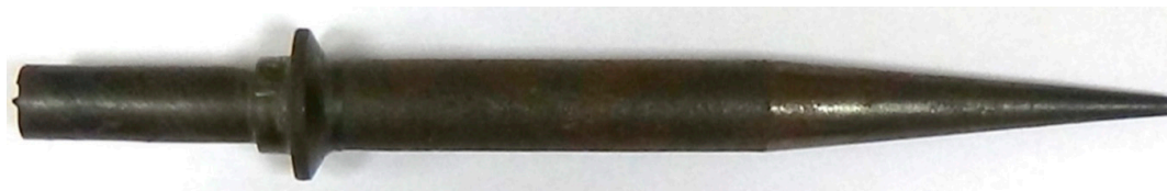
Figure 5. Preform of the harrow tooth obtained in the researched CWR process.
