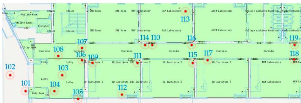
Figure 8. Indoor Map and the approximate position UWB anchors on the first floor of the building.
