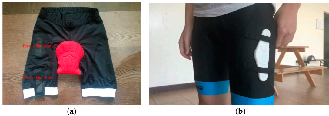
Figure 12. (a) Photo of the lining of the bicycle pants; (b) the EMG patch was placed on the bicycle pants to measure the lateral femoral muscle.
