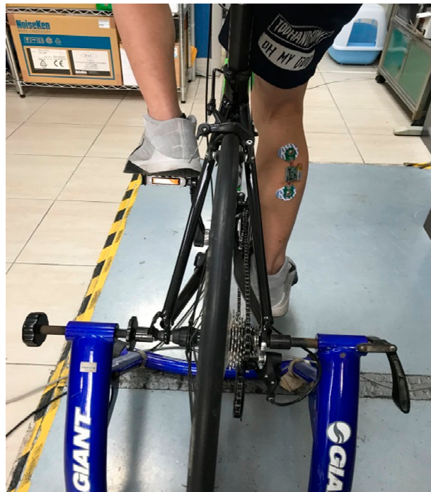
Figure 7. A photo of the experimental EMG patch.
