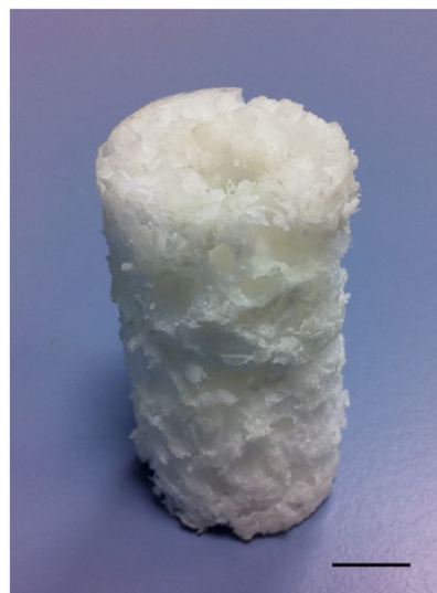
Figure 1. Binary polymer scaffold following processing; note the longitudinal intramedullary canal; scale bar = 10 mm. [Colour figure can be viewed at wileyonlinelibrary.com ]
