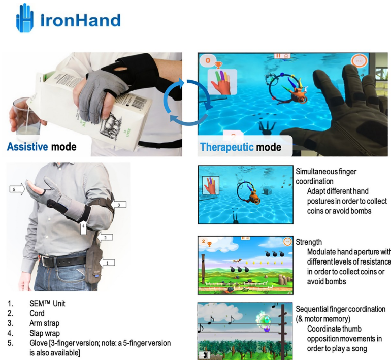
Fig 2. Overview of the ironHand system with assistive functionality (left panel) and therapeutic functionality (right panel). * Reprinted from Bioservo Technologies under a CC BY license, with permission from Bioservo Technologies, original copyright 2017.
