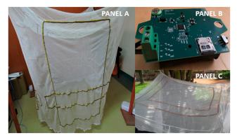
FIGURE 1. SmartNet components: (A) Slide view of unfurled SmartNet; (B) SmartNet battery-powered microcontroller; (C) Top view of SmartNet. This figure appears in color at www.ajtmh.org.
