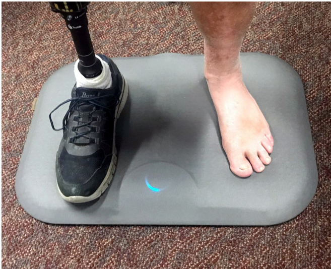
Figure 1 The study device is a daily-use telemedicine mat with integrated thermometric sensors and secure transmission of data via cellular network for analysis and triage.
