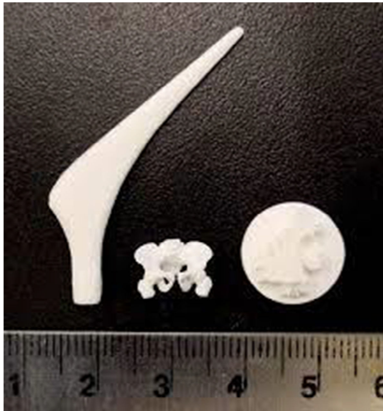
Fig. 42. Hip stem, human pelvis and WSU logo printed by binder jetting 3D printer using TCP [94].
