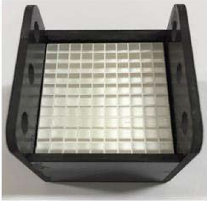
Fig. 7. 10 × 10 array of 3 mm × 3 mm × 20 mm LYSO scintillator crystals for the one-to-one coupled detector experiments.
