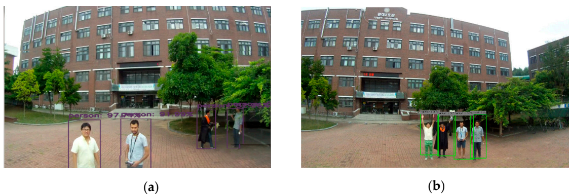
Figure 16. Target detection results from the drone of (a) YOLO tiny using Odroid XU4 + NCS and (b) SSD-MobileNet using Odroid XU4 + NCS.
