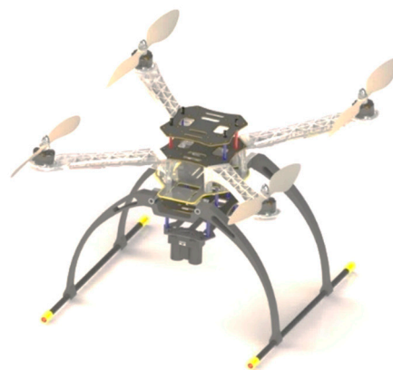
Figure 1. 3D CAD design of the external structure of an aerial vehicle with a camera mounted on it.
