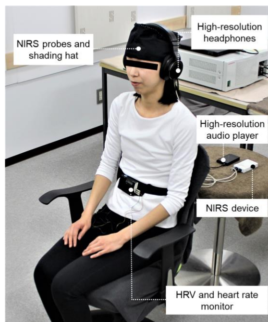
Figure 1. Experimental set-up for auditory physiological measurement. NIRS: near-infrared spectroscopy; HRV: heart rate variability.
