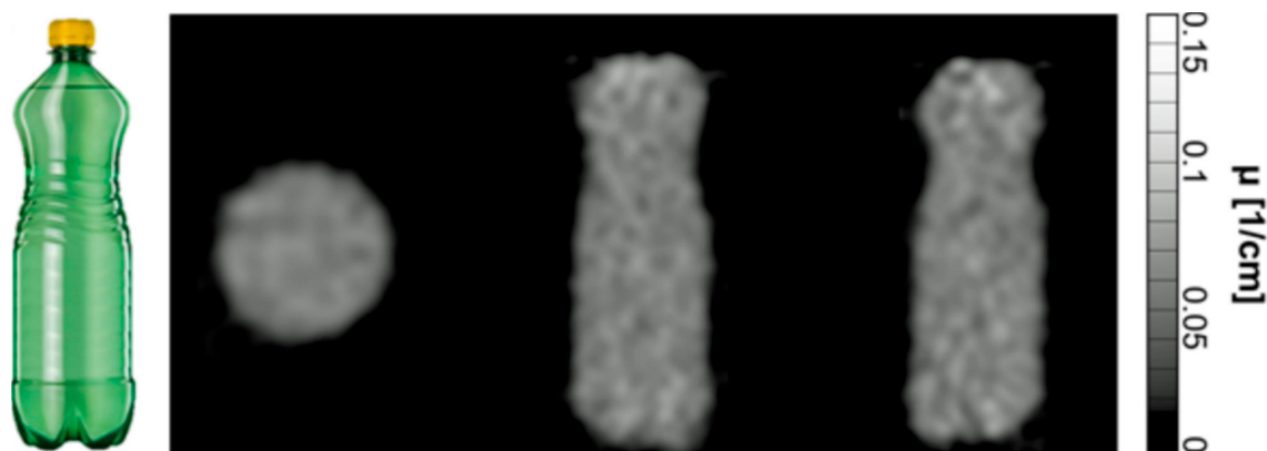
Figure 10. PET attenuation map. Left: Water bottle (1 L) used for the first PET AC calculations. Right: Reconstructed attenuation maps in all three directions using acquired data from the transmission scan.
