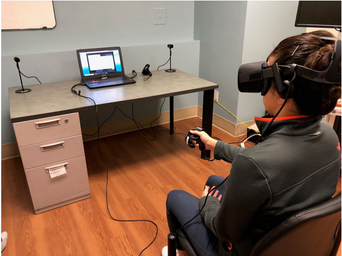
Figure 1: System setup for individual with left hemiplegia including laptop computer, tabletop sensors, headset and controller.
