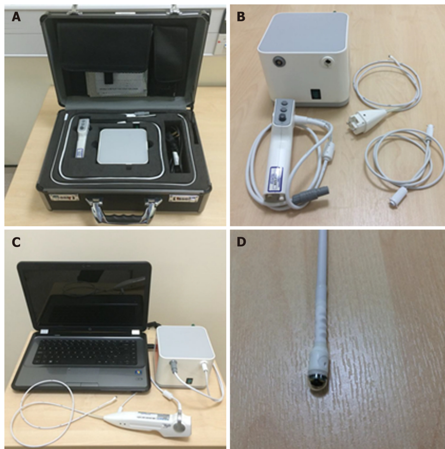
Figure 1 The “EG Scan II” system. A: The portable case with four main parts; B: The image processor (top left), disposable probe (top right), air tube (bottom right) and hand-held controller (bottom left); C: The system connected and ready for use; D: Close view of the capsule probe tip. Reproduced with permission from Sami SS et al. Copyright John Wiley and Sons.
