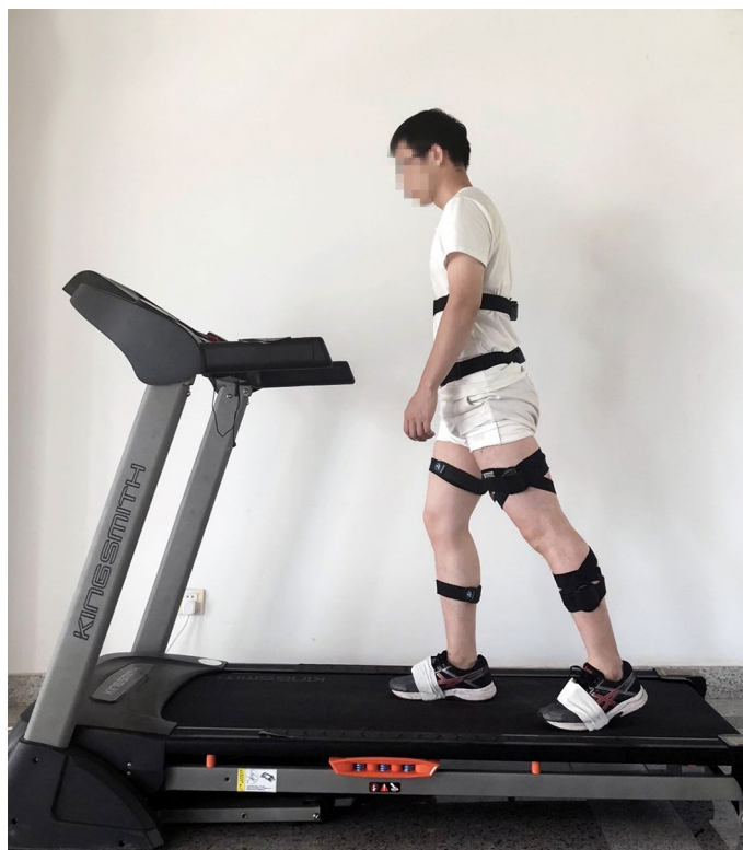
Fig. 6 Motion capture experiment in treadmill walking. The IMU and EMG sensors were attached on the subject's body. The data was transmitted to the computer wirelessly
