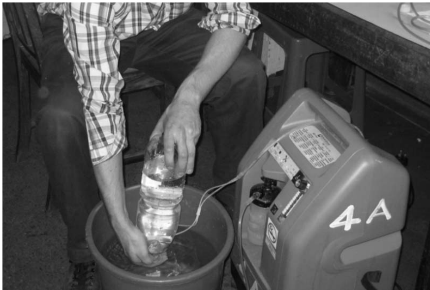
Figure 1 Photograph demonstrating technique used to assess oxygen flow from an oxygen concentrator.
