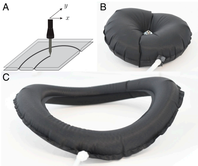
Fig. 1. Flat sealed inflatables. (A) Heat sealing of 2 sheets together along a desired path using a soldering iron mounted on a 2-directional plotter. (B) Photograph of an experimental realization of inflating an annulus of inner radius R and width w , with R/w \rightarrow 0 . Wrinkles appear, and 2 diametrically opposed kinks are observed. (C) For R/w \gg 1 , the inflated structure buckles smoothly out of plane. Both structures are made of thermoplastic polyurethane-coated nylon fabric.
