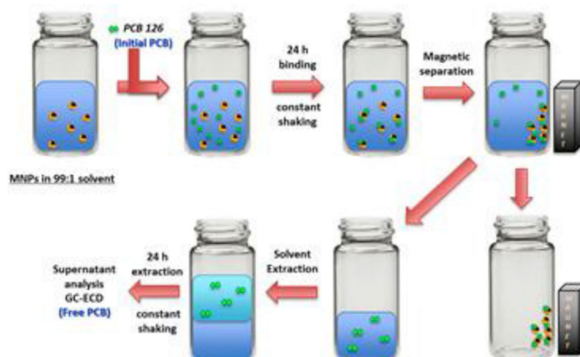
Fig. 1. Schematic representation of the binding studies conducted with PCB 126 in a 99:1 DI water ethanol solvent.
