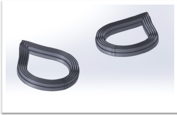
Fig. 1. CAD image of an example of one of the flat seal samples. This particular sample has soft ribs that are designed to penetrate through the facial hair as much as possible while still remaining comfortable for the wearer. Brought together, which creates a chamber with the flat seal sample pressed against the simulated facial hair surface at the joint of the two halves. Air can then be introduced to the closed chamber via a tube to assess how well the seal maintains air pressure inside the chamber. A corresponding tube is connected to the chamber to take pressure readings.
