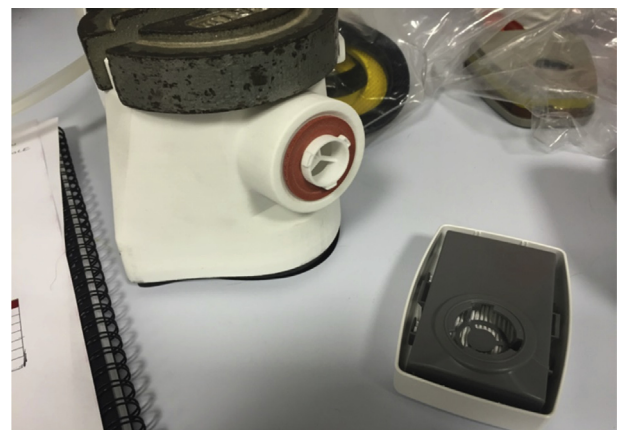
Fig. 16. New filters presented by the ITL, note standardized fitting detail.
