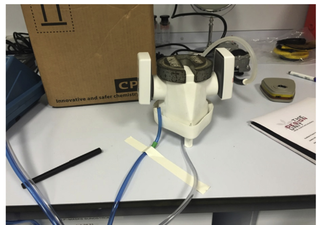
Fig. 15. The test rig connected to the PortaCount machine: the blue tube measures particulate outside the test rig chamber, the clear tube at the front of the test chamber measures the test chamber inside and is connected to the PortaCount machine, and the clear tube at the rear end of the photograph is connected to the vacuum pump which draws air through the filters and into the test chamber.
