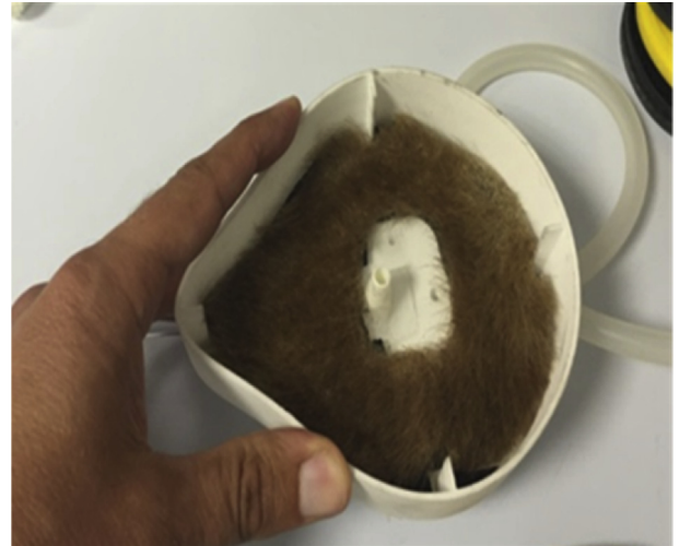
Fig. 3. Bottom cup, housing facial hair sample mounted on a soft substrate.
