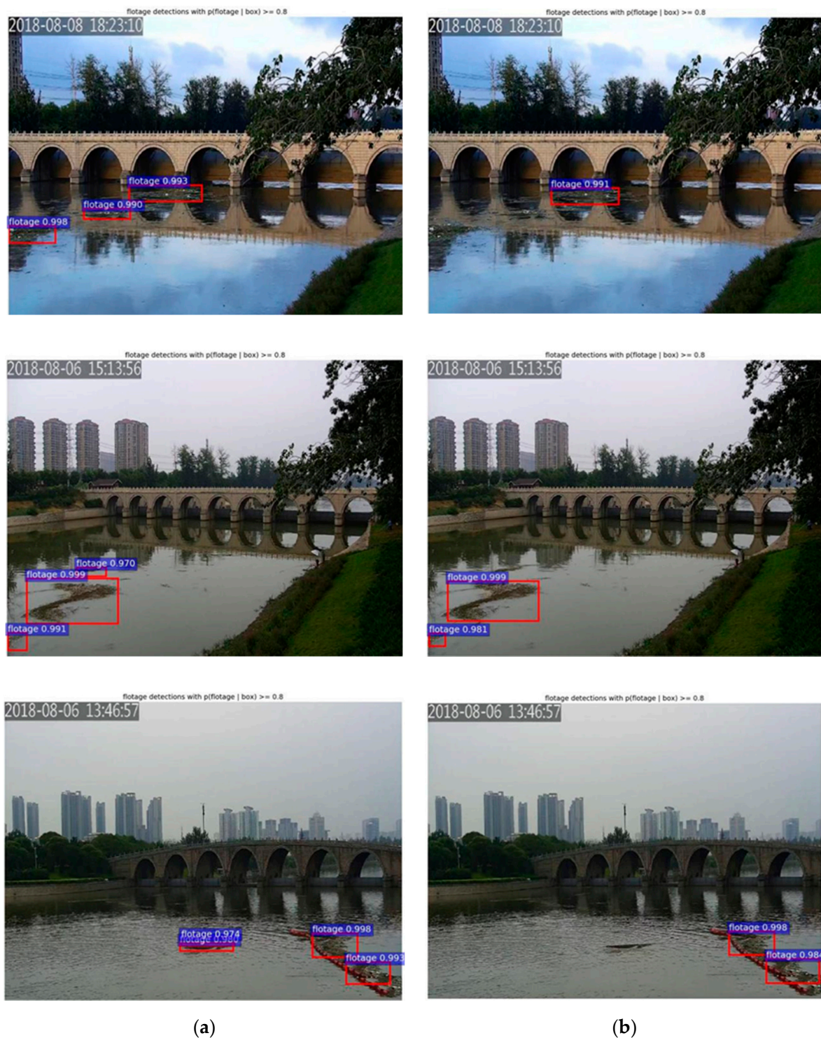
Figure 8. Detection results of Faster R-CNN (a) with and (b) without feature fusion.
