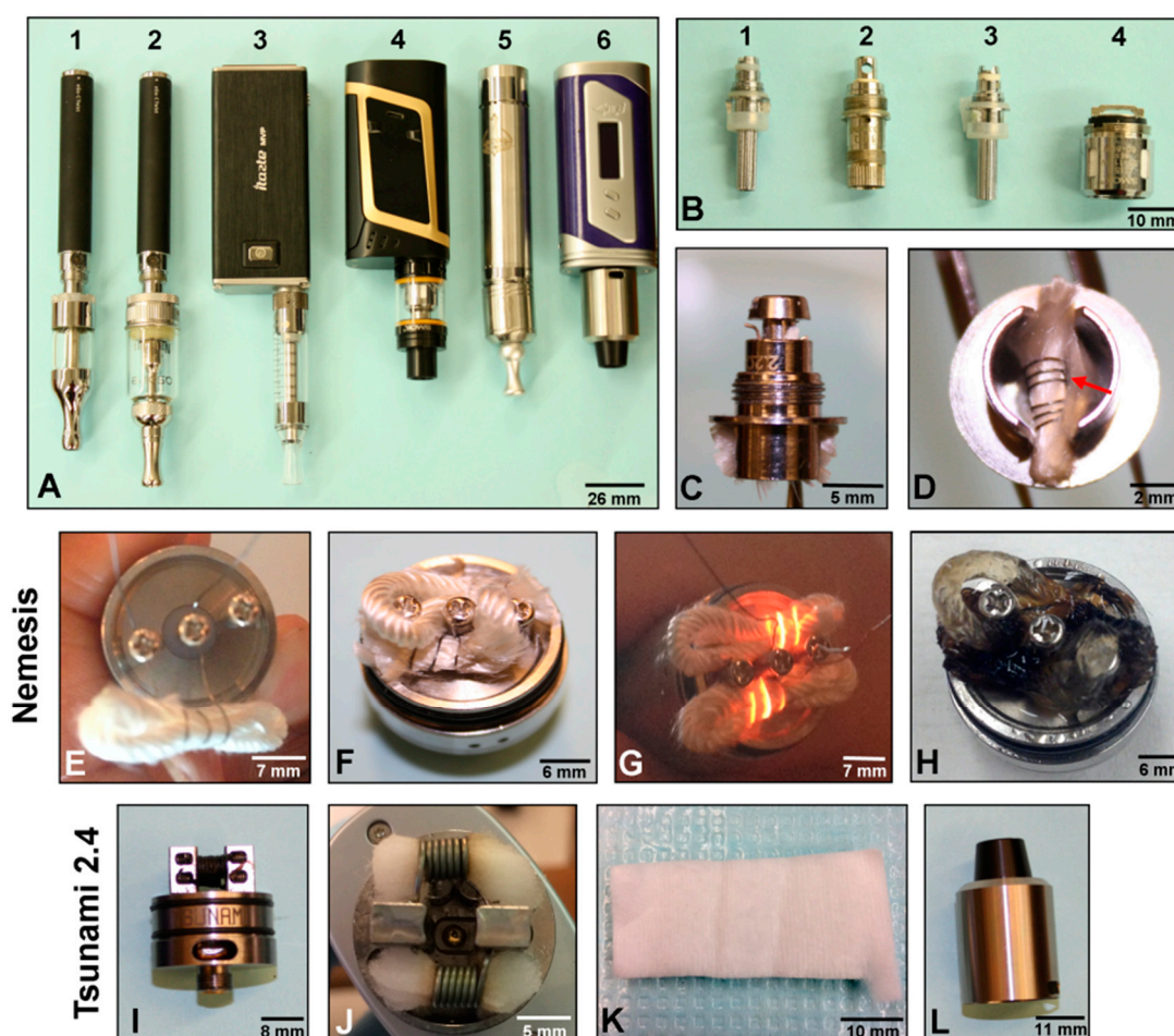
Figure 5. Comparison of batteries, reservoirs, and atomizing units in different models of second and third generation clearomizer/mod-style ECs. (A) Layout of all batteries and reservoirs used in the study: 1 (Ego C Twist, Kangertech Protank), 2 (Ego C Twist, Aspire Nautilus), 3 (iTaste MVP, Kanger T3S), 4 (Smok Alien, Smok), 5 (Nemesis, Clone), 6 (iPV6X, Tsunami 2.4). (B) Atomizing coils from left to right for 1 (Protank), 2 (Aspire), 3 (Kanger T3S), 4 (Smok). (C) Profile of top of the atomizing coil from Protank. (D) The wick and filament (red arrow) from Protank. (E) Partially built coil from Clone RDA. (F) Fully built Clone atomizer with two coils and wicks. (G) Testing the coils were properly built in the Clone atomizer. (H) Appearance of the coils from Clone atomizer following 60 puffs. (I) Side profile of the Tsunami atomizer. (J) Fully built Tsunami atomizer with wicks. (K) Detail of the wick for the Tsunami atomizer. (L) Cap for covering the Tsunami atomizer.
