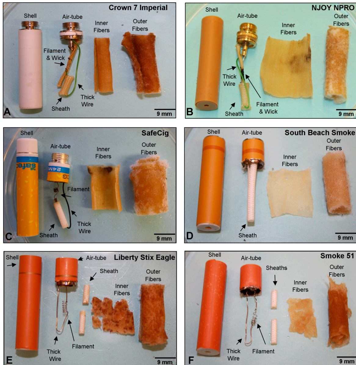
Figure 3. Anatomy of atomizers from cartomizer style ECs showing three different design categories. (A) Crown 7 Imperial, (B) NJOY NPRO, (C) SafeCig, (D) South Beach Smoke, (E) Liberty Stix Eagle, (F) Smoke 51. The shell, air-tube, filament, wick, sheath, thick wire, and inner and outer fibers are labeled in (A). Design category 1 (A–C), category 2 (D), and category 3 (E–F).
