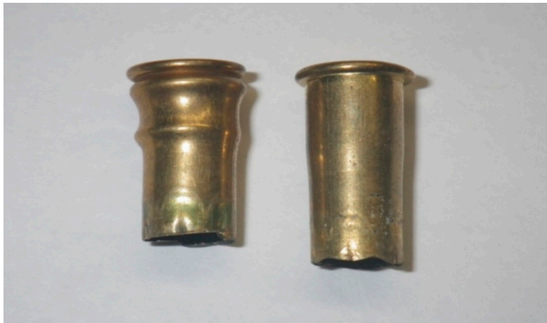
Figure 17. Deviation of cases fired in the same device. Right hand case displaying rim end expansion as expected to seal the case within the breech; left hand case showing deformity and signs of having moved backward on firing.
