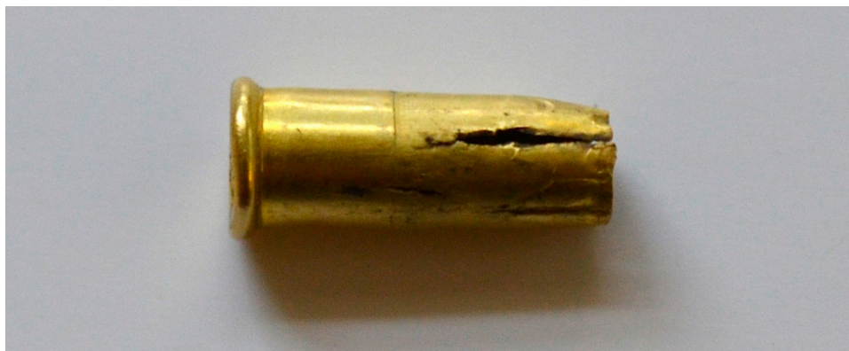
Figure 19. Case splitting in an AS head stamped 0.22” calibre cartridge.
