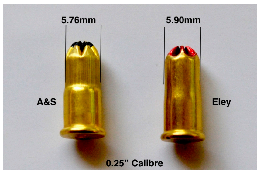
Figure 21. Variation in case diameter between AS and Eley cartridges for use in the same 0.25" calibre device.
