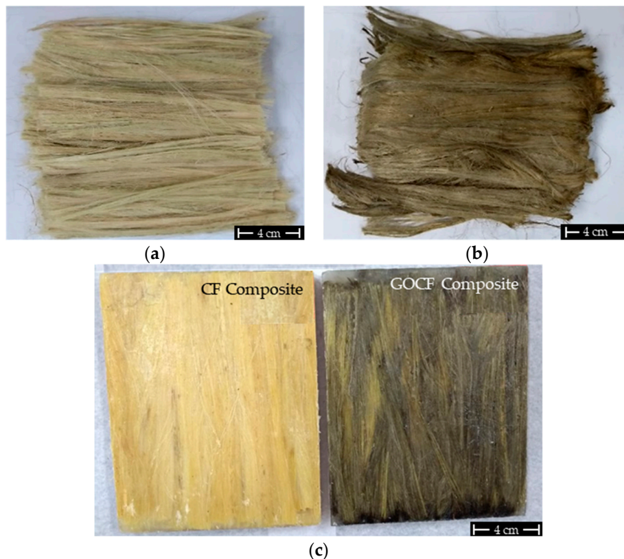
Figure 1. General macroscopic aspect of curaua fibers: (a) curaua fibers (CF); (b) graphene oxide coated fibers (GOCF); (c) their 30 vol% epoxy composites.
