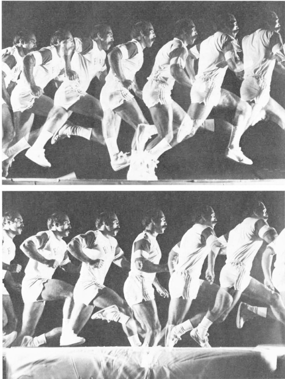
Figure 7. RUNNING FILMS show that whether a runner is on a fairly stiff wood track ( top ) or on a soft pillow track ( bottom ) the trajectory of his head is nearly level. Therefore for the purposes of the model it can be assumed that the hip follows a level path no matter what surface runner is on. Assumption simplifies calculation of effect of track stiffness on the step length ( see bottom illustration on opposite page ).
