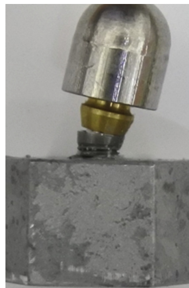
Figure 8 3i internal hex implant system after loading. Gap formation over fixture abutment interface was noted.
