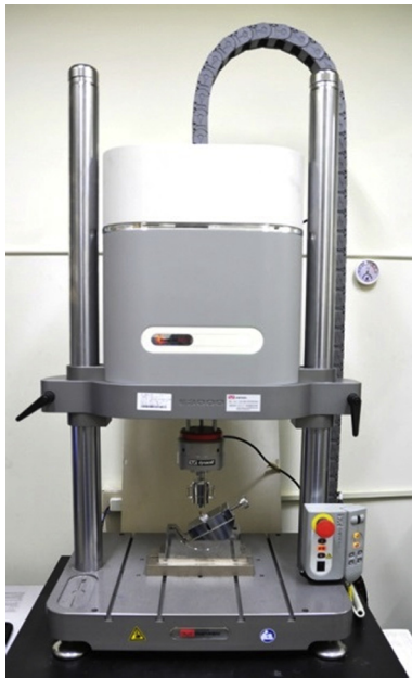
Figure 5 Instron E3000 with axial load cell (Instron, Canton, MA, USA).
