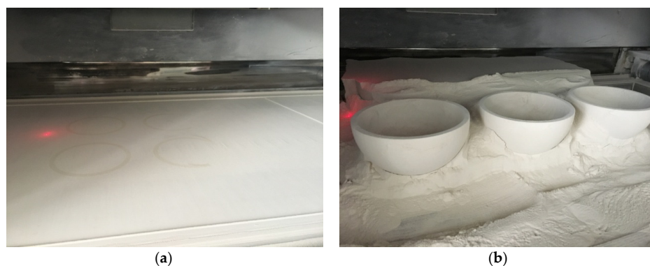
Figure 3. (a) Printing the hemispherical greenbodies in the additive manufacturing (AM) equipment, and (b) the printed hemispherical greenbodies.
