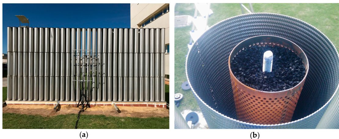
Figure 1. Sonic crystal (SC) barrier sample implemented on the campus of Universitat Politècnica de València: (a) Appearance of SC barrier sample made of three rows of absorbing cylindrical units, along with experimental setup; (b) internal cross-section of a cylindrical unit, consisting of a porous core made of rubber crumb and outer micro-perforated aluminium shell.
