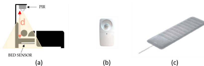
Figure 1. (a) The measurement set-up during the test nights with the user lying in bed and the Passive InfraRed PIR sensor installed at a distance d of 1.10 m above the pillow; (b) PIR sensor; (c) reference bed sensor (Nokia sleep bed sensor) installed under the mattress.
