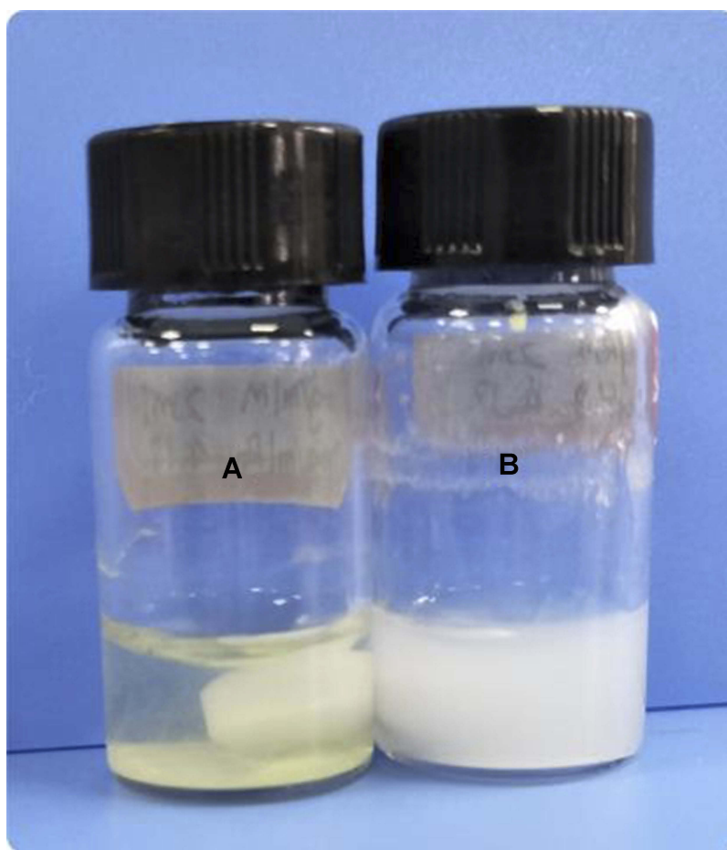
Figure 1 Formation of a colloidal suspension of RADA16-I and mangiferin (MA). (A) MA with pure water. (B) MA with RADA16-I. The photograph was taken after the mixture was magnetically stirred for 24 h. [MA]=0.5 mg/mL, [RADA16-I]=5 mg/mL.
