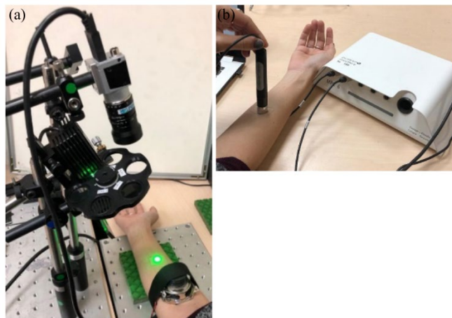
Fig. 2. The two experimental instruments: (a) Our optical setup, extracting the optical parameter. (b) The Corneometer CM 825 probe (by Courage + Khazaka, Germany) measuring capacitance.
