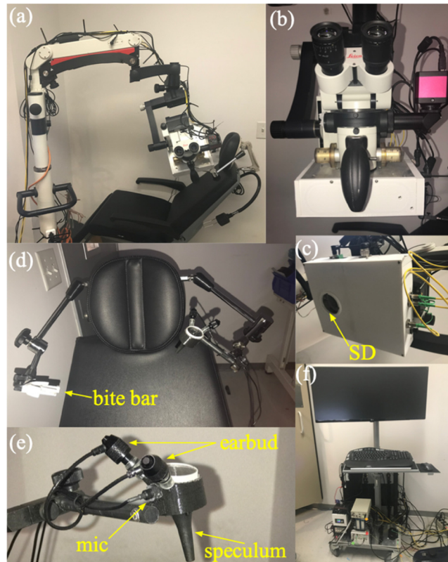
Fig. 2. (a) Leica M400E surgical microscope with OCT accessory attachment and ENT examination chair. (b) Close-up showing the OCT accessory mounted to the bottom side of the microscope. (c) Bottom view of OCT accessory. The bottom cover is threaded to match the sterile drapes (SD) commonly used to cover the microscope when used in surgery. (d) Close-up of ENT chair head rest showing the bite bar on the left used for high-phase sensitivity measurements. The speculum fixture is on the right. Both are attached to the chair with lockable articulating arms. (e) Close-up of speculum fixture showing the two earbuds used for introducing sound to the ear canal, the microphone for recording the stimulus sound, and a disposable speculum. (f) Mobile tower, housing the CPU, monitor, all electronics, laser system, and detector.
