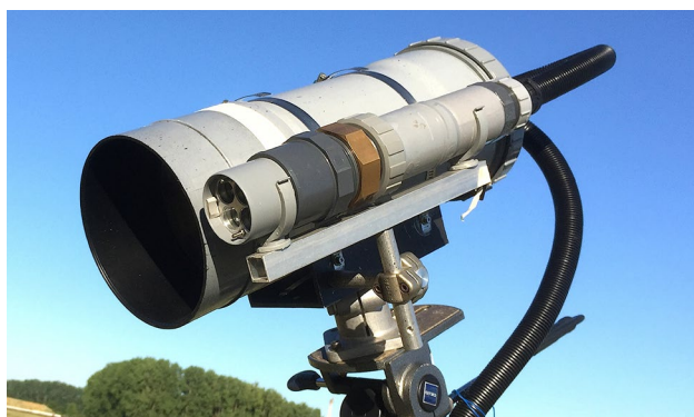
Fig. 1 The LEDFLEX micro-lidar. The smaller tube contains the excitation source and the driver electronics. The larger tube contains the detection optics, the detector and its amplifier, the acquisition board, and the computer
