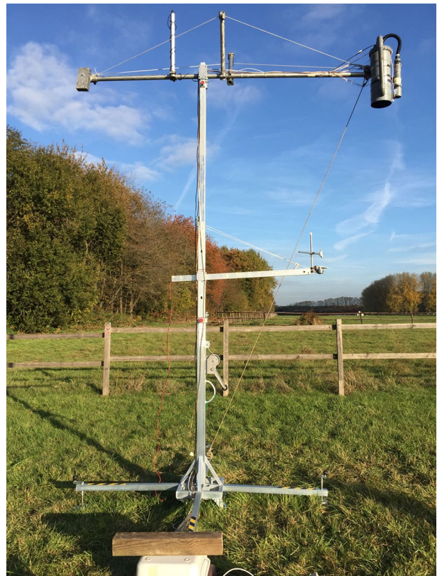
Fig. 5 LEDFLEX in operation above grassland. The PAR sensor is fixed on a vertical rod above the boom. The boom is rigidified with ropes to avoid any movements due to wind
