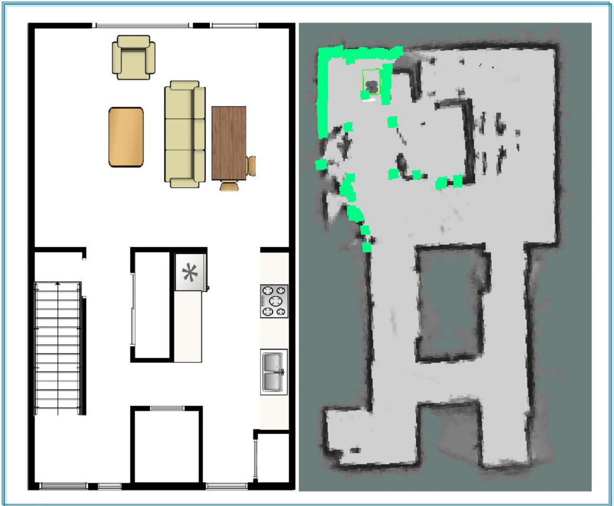
Figure 5. (left) Smart home floorplan. (right) Cartographer-generated home map. Green dots indicate current LiDAR scan.
