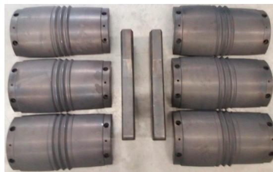
Figure 13. A set of segmented tools with helical passes for rolling rods from scrap rail heads.
