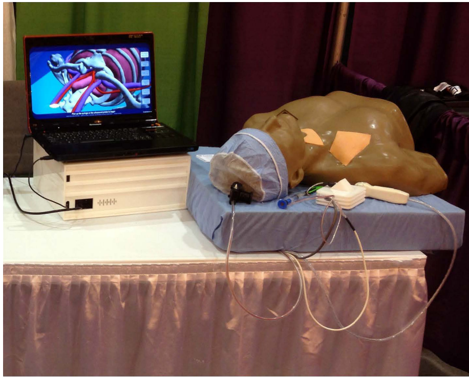
Figure 1. The mixed reality simulator of central venous access used in the study. The three-dimensional visualization is displayed on the laptop screen.
