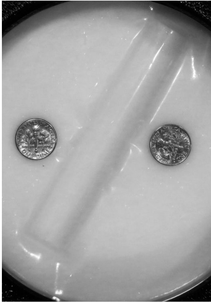
Fig. 1. One of the reference phantom surfaces showing the slot in which one of the transvaginal transducer probes is positioned in order to obtain a full-field B-mode image (as well as the raw RF data). Scale: a US coin (dime) has a diameter of 1.8 cm.
