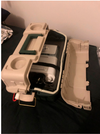
FIGURE 3. (A) C-Box to place the continuous positive airway pressure (CPAP) machine. (B) Showing CPAP machine placed inside the C-Box. (C) Showing CPAP machine placed inside the C-Box while in use. This figure appears in color at www.ajtmh.org .
