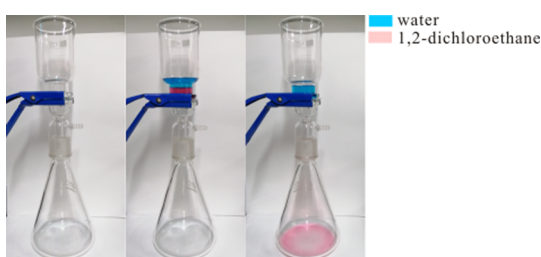
Figure 13. Oil–water separation process of copolymer–SiO 2 NPs/PDMS-coated paper (taking 1,2-dichloroethane as an example).
