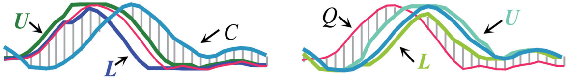
Fig. 10. (left) Normally the LB_{Keogh} envelope is built around the query (see also Figure 6(right), and the distance between C and the closer of \{U, L\} acts as a lower bound (right). However, we can reverse the roles such that the envelope is built around C and the distance between Q and the closer of \{U, L\} is the lower bound.
