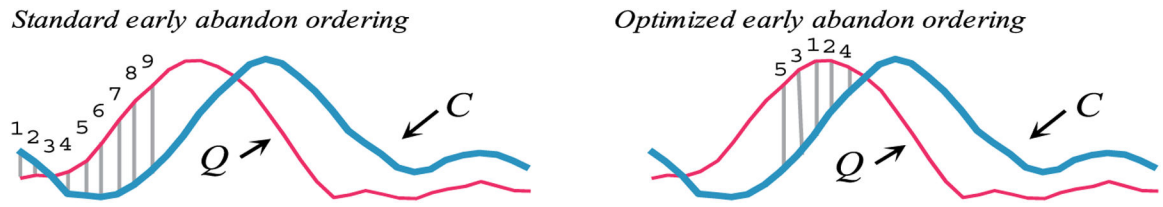
Fig. 9. (left) ED early abandoning . We have a best-so-far value of b . After incrementally summing the first nine individual contributions to the ED, we have exceeded b , thus, we abandon the calculation. (right) A different ordering allows us to abandon after just five calculations.
