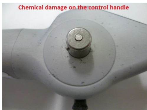
Figure 5 Inadequate drying following sterilisation can result in chemical damage to the hand-piece.
