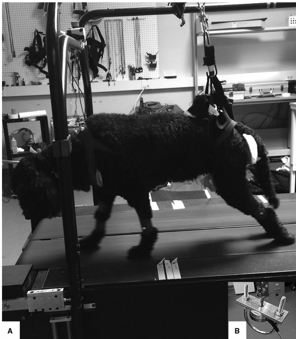
FIG. 1. (A) Set-up for dogs with spinal cord injury on the instrumented treadmill depicting sling support attached to the load cell and reflective marker placement. (B) Close-up view of load cell.
