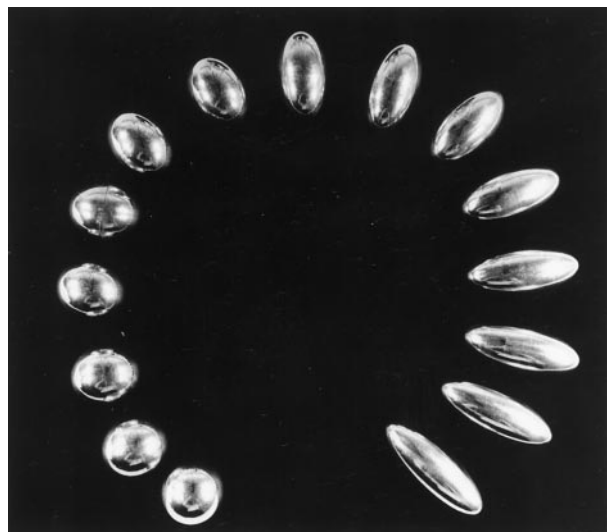
Figure 1. The fifteen spherical ellipsoids. The fifteen ellipsoids used in this experiment were made to have the same weight and surface, differing by their shape only. Two similar sets were used.
