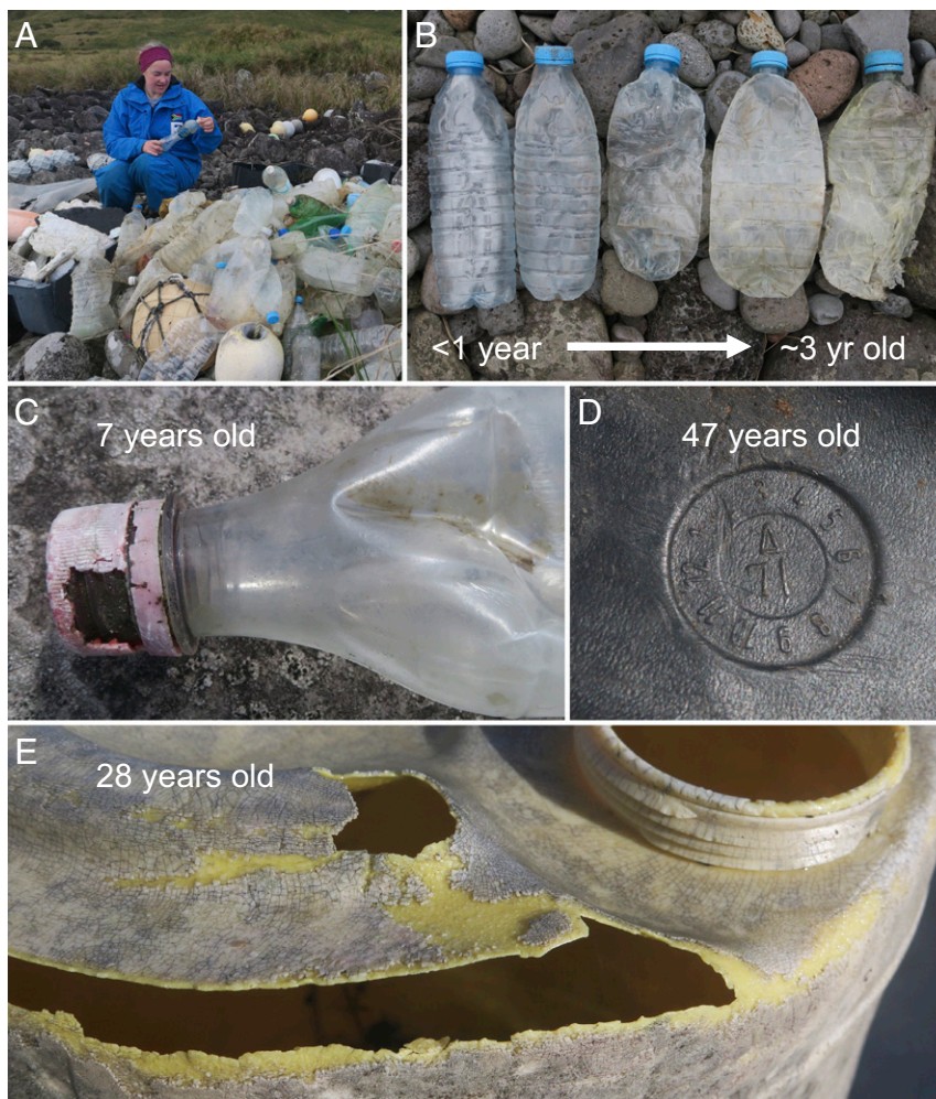
Fig. 2. (A) Checking cached bottles for manufacturers' marks on Inaccessible Island. (B) Mechanical wear on Master Kong 500 mL water bottles over the course of roughly 3 y. (C) A soft drink bottle with a stamped date of April 2011 showing UV damage to the HDPE lid. (D) The date stamp on the oldest item found, an HDPE canister made in March 1971. (E) A 20-L canister manufactured in November 1990 showing surface crazing and embrittlement characteristic of UV degradation.
