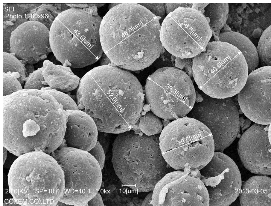
Figure 17 SEM demonstrating CaHA filler particle size as 36–52 microns at 1000× magnification. Particles had smooth surfaces, were completely spherical, and had about 3-micron-sized small holes in the surface.
