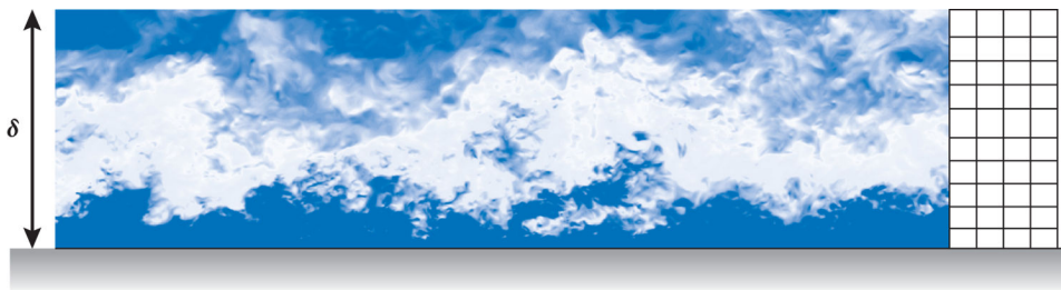
Figure 2. Schematic illustrating a typical wall-modeled grid resolution, chosen to resolve the energetic eddies in the outer portion of the boundary layer, whose size scales with \delta . Contours visualized represent the instantaneous streamwise velocity in a turbulent channel flow ( Re_\tau = 4,200 ). The contours range from U^+ = 6 ( blue ) to 18 ( white ). Data taken from the direct numerical simulation of Lozano-Durán & Jiménez (2014); reproduced with permission, courtesy of A. Lozano-Durán.
