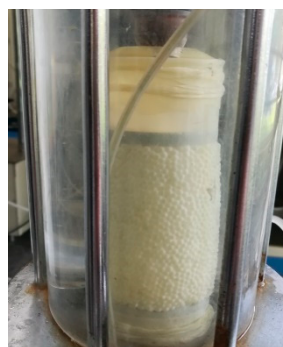
Figure 9. Glass bead specimen in triaxial test.
