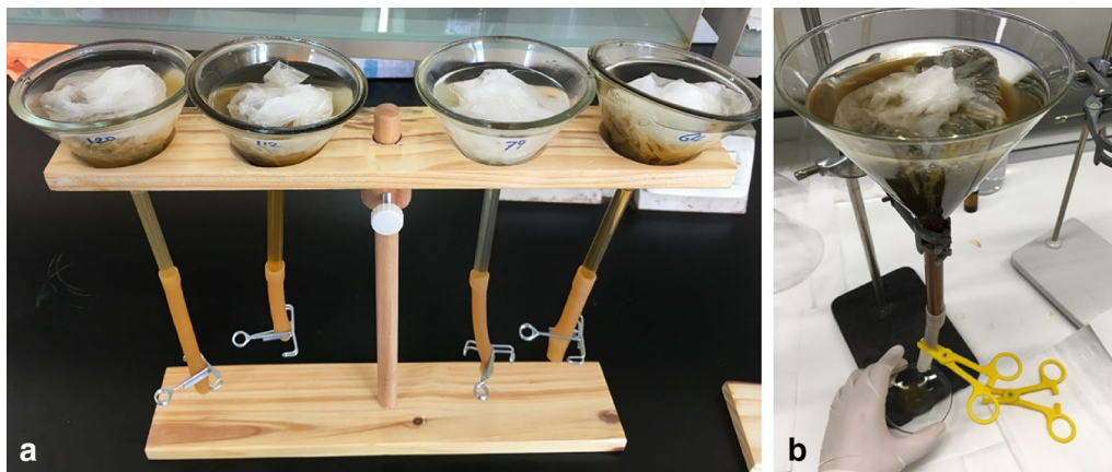
Fig. 4 a Baermann funnel set up. b Worm harvest from the Baermann funnel
