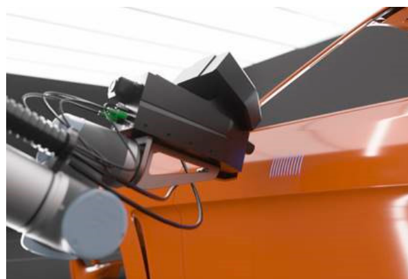
Figure 12. Implementation of a THz TDS in an industrial setting. Courtesy of Helmut Fischer GmbH.
